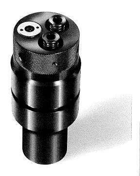
more axial clamping depends on the cutter arbor and is supervised by the clamping pressure indicator. The clamping pressure is reached as soon as the red ring indicator pin reaches the height of the golden insert. There exist no transverse forces causing a shifting on the hobbing cutter.
