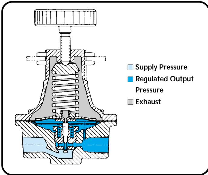
Figure 1. GH10 Series. Bleed and Relief Diaphragm
