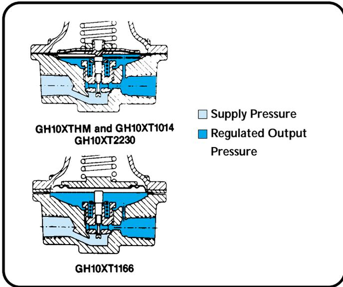
Figure 2. GH10 Series. No Bleed/No Relief Diaphragm
