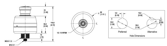
Figure 2. Standard 40 mm Pushbutton
