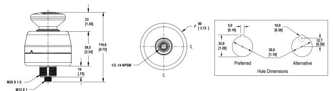
Figure 3. Large 60 mm Pushbutton
