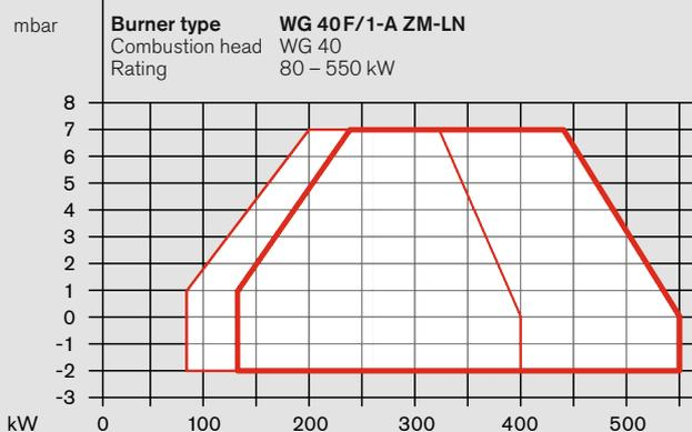
Combustion head open ——— Combustion head closed ———
