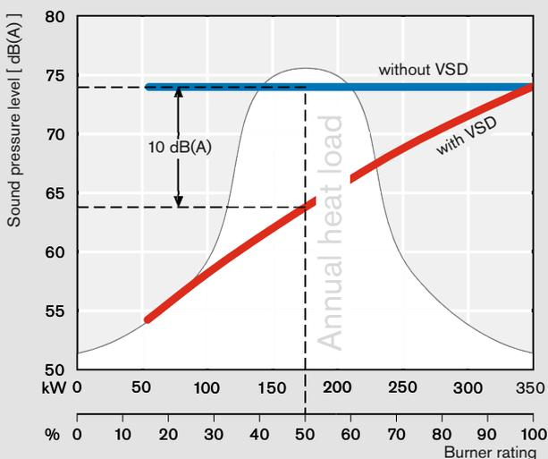
Typical reduction in sound pressure level for a WG30 gas burner
