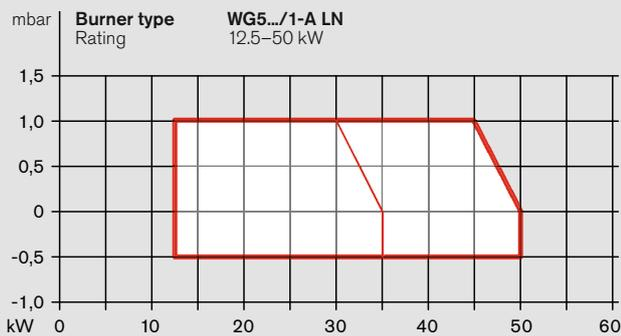
Combustion head open ——— Combustion head closed ———
