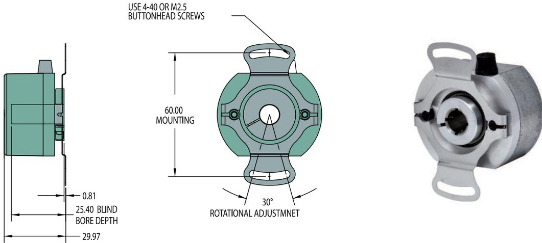
All dimensions are in mm with a tolerance of  $\pm 0.127\text{mm}$  or  $\pm 0.254\text{mm}$  unless otherwise specified
