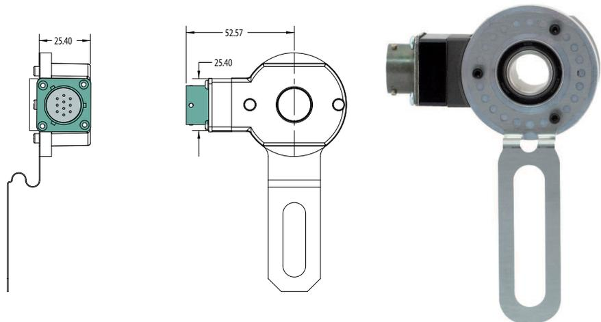
All dimensions are in mm with a tolerance of ±0.127mm or ±0.254 unless otherwise specified
