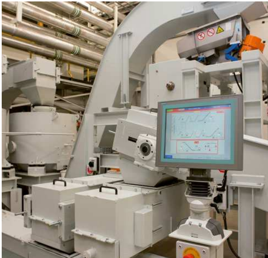
VBU swarf centrifuge for continuous use
