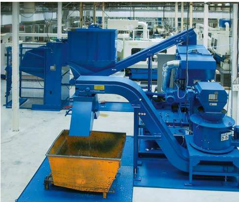
Swarf pressing system comprised of the following components: centrifuge, swarf crusher, conveyor and container loading
