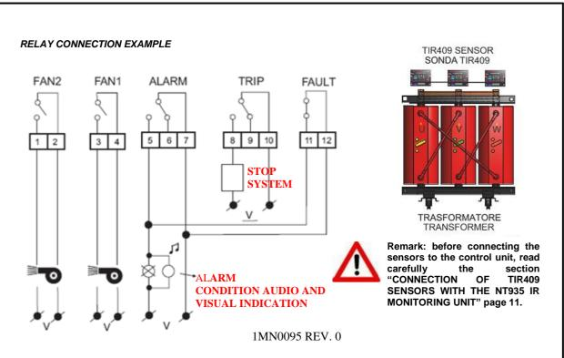
Output relay with 10A-250Vac-res COS $\Phi$ =1 contacts.
