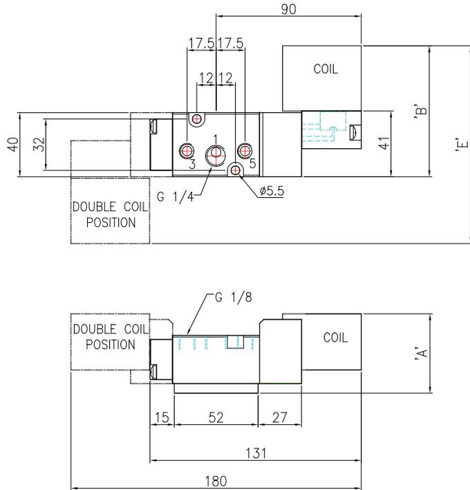
The coil itself can be rotated in 90° steps by releasing the four securing screws. (FIG 3) When rotating the coil care should be taken to ensure the core assembly (core, spring, seal and washer) remains intact and aligned correctly. This is easily achieved by only lifting the coil the small amount required to clear the screws enabling the coil to be rotated.
