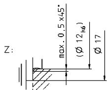
Non-toleranced dimensions  $\pm 1\text{mm}$
