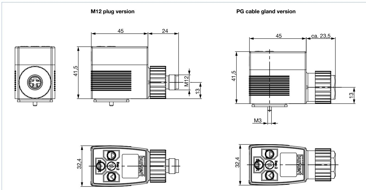
Cable plug without control unit (analogue and bus versions, for bus version only M12 plug, 5-pin)
