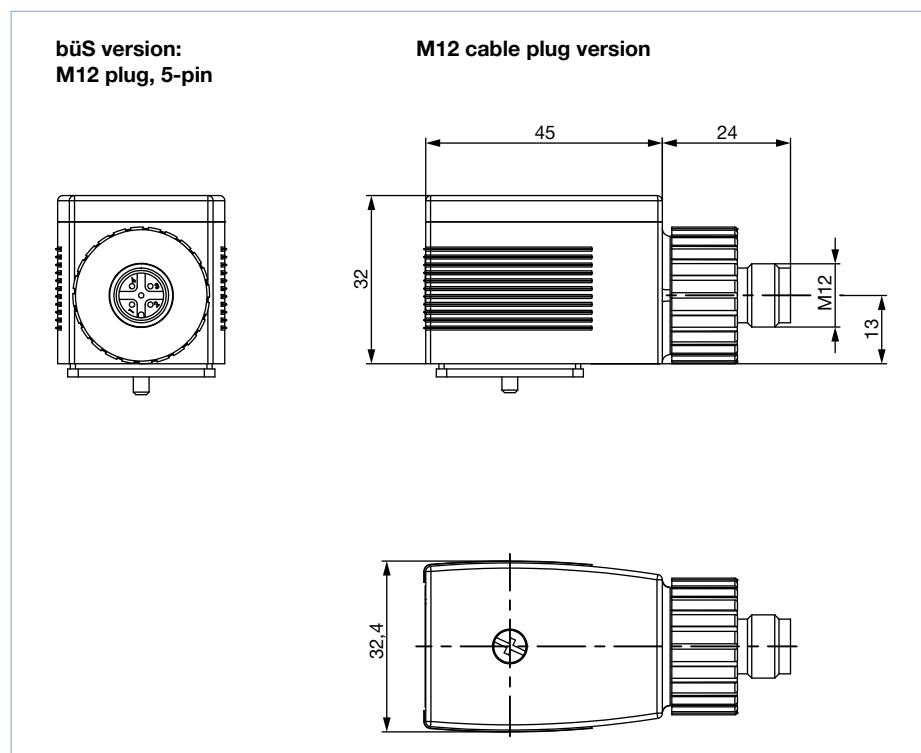
**Cable plug M12 male connector, 5-pin and sensor input M12 female connector, 5-pin**
