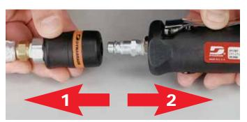
Step One: Pull back on the sleeve and the compressed air is vented.
