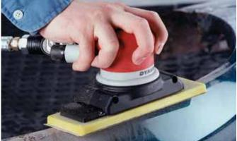
On Non-Vac Model, Pad Can Be Rotated 360° and Set at Any Comfortable Position. No Other Tool Like It!
