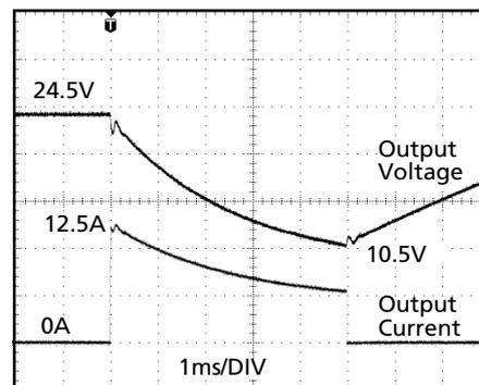
Peak load 12.5A (resistive load) for 5ms
