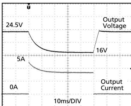
Peak load 5A (resistive load) for 50ms
