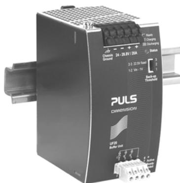
The buffer unit does not require any control wiring. It can be added in parallel to the load circuit at any given point. Buffer units can be added in parallel to increase the output capacity or the hold-up time.
