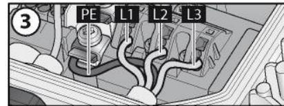
Fig. 2: Connecting wires to terminals
