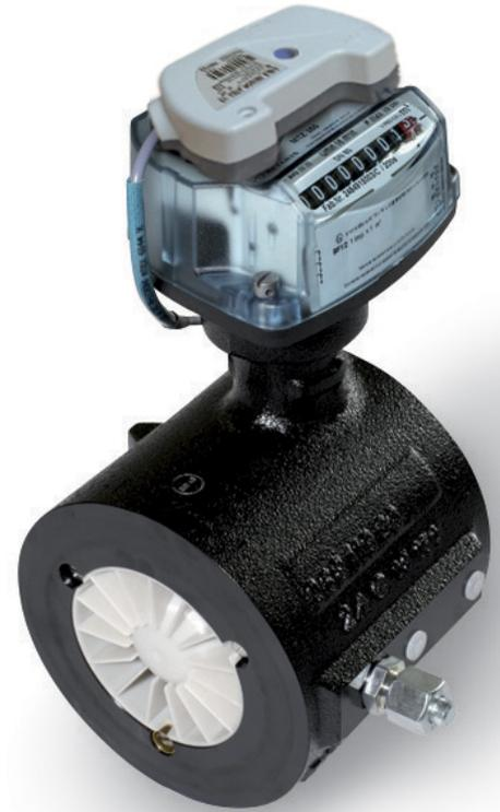
MZ meters are flow meters. The flow of gas turns the turbine wheel, and thus the rotating speed of the turbine is proportional to the linear speed of the gas. The movement is mechanically transmitted to the totaliser through a magnetic coupling.
