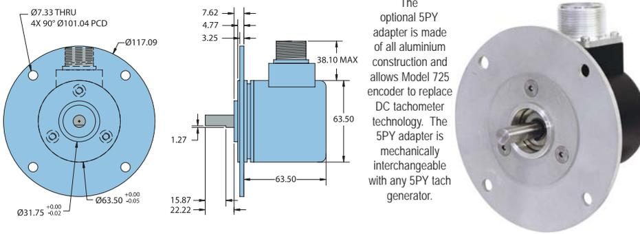
The optional 5PY adapter is made of all aluminium construction and allows Model 725 encoder to replace DC tachometer technology. The 5PY adapter is mechanically interchangeable with any 5PY tach generator.
