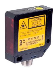
reflection sensor, the transmitter and receiver are in one device. The emitted light beam is reflected by the object that is to be detected. As soon as the receiver detects the reflected light, the switching output integrated in the device changes its status.
