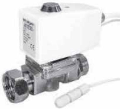
In case of leakage, a sensor activates a solenoid valve to shut down the water supply. Included is a controlling device, solenoid valve and 5 m connection cable. Applications include, water and neutral or electrically conducting fluids.
