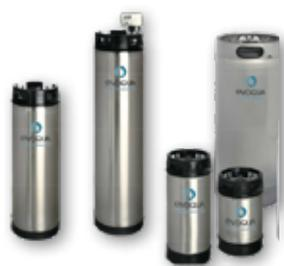
Mixed bed resin ion exchangers are used to generate demineralized water. These high-quality stainless steel ion exchangers (1.4404) can be operated with a working pressure of max. 10 bar. Our optimized channel flow ensures superior resin bed usage. The cartridges are available optionally with the proven stainless steel quick couplers (SK) or with threaded fitting (3/4" / 1 1/4"). Conductivity meters and tubing (or electrodes) are available separately.
