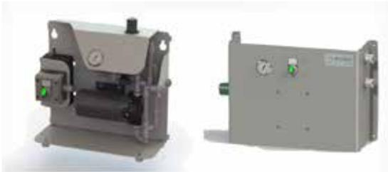
Evoqua pressure booster systems are ready-to-be-installed water supply systems consisting of a self-priming membrane pump with an overflow valve, a pressure reducer to set the working pressure with a manometer, and a simple On/Off automatic switch.
