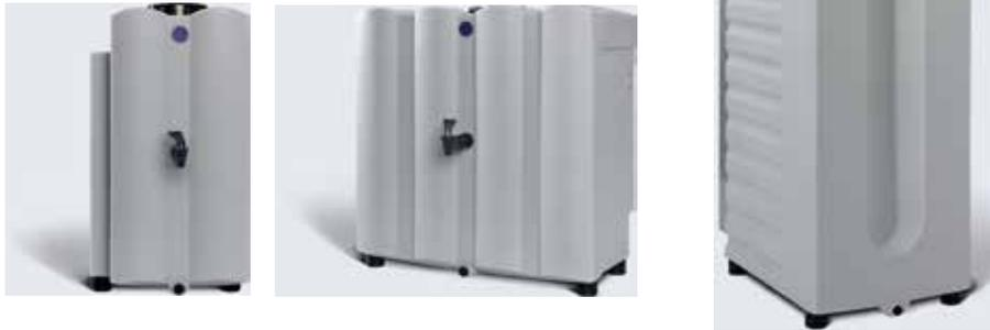
Storage tanks with conical bottom for pure water are constructed from polyethylene to minimise the release of organics. Vent filters prevent the ingress of airborne impurities. Further accessories see below. Level control with pressure sensor (4 - 20 mA).
