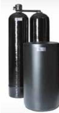
These fully automated, quantity-controlled, mechanical twin water softening systems offer, among other aspects, continuous availability of soft water with low salt and water consumption and very easy installation. Thanks to its synthetic components the system is non-corroding. The systems are monitored with a hydraulic control button. Therefore, a Power supply is not required. The systems are powered para flow and ensure maximum reduction of hardness with full use of volume capacity.
