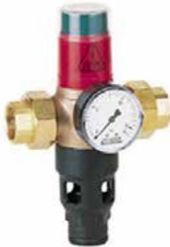
DIN/DVGW validated to protect potable water supply from contamination due to backflow. The brass casing has screw fittings on either side and spouts with internal threads. Backflow protectors are made of high-quality synthetic material. Included is a pressure gauge and a hopper for attachment of a 40 mm plastic pipe or R 1" threaded pipe.
