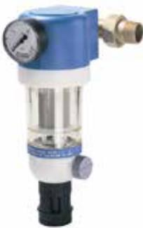
Backflush filter and washable fine filter for water. Validated according to DIN/DVGW (German Technical and Scientific Association for Gas and Water). The fine filter is made from stainless steel. Backflushing is conducted with filtered water over the entire filter surface, without interrupting the water supply. After opening the ball valve, all particles and the backflush water are flushed out automatically and completely.
