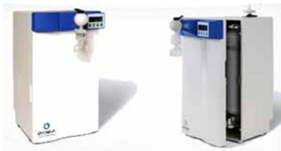
The extremely space-saving ultrapure water system for cost-efficient generation of analytical-grade water can be used as a benchtop device. The water quality with a conductivity of 0.055 µS/cm corresponding to 18.2 MΩ-cm and a TOC content of < 10 ppb in the DI version and 1 - 5 ppb in the UV version exceeds all standards, such as: ASTM type I, CLSI type I and ISO 3696 type I.
