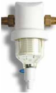
Rinsing fine filter to protect water according to DIN/DVGW (German Technical and Scientific Association for Gas and Water) from coarse particles or other undissolved materials from the drinking water network. The housing is made from high-quality synthetic material. Rinsing with untreated water occurs over the entire filter surface without interrupting water supply. After opening the ball valve the particles are flushed out automatically and completely through the built-in drain outlet.
