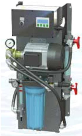
The RO 100 Easy is a cost effective, efficient and compact reverse osmosis system producing 100 L permeate per hour from drinking water. The system can be wall or bench mounted, with direct access to all spare parts. Applications include glass washers, autoclaves and applications requiring Type III water.
