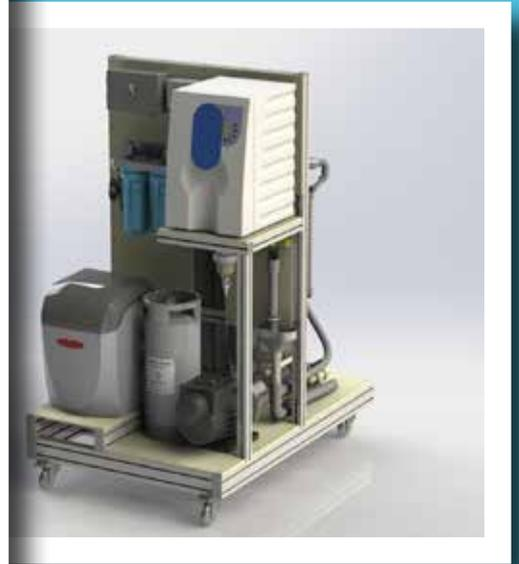
1. Central water treatment system, consisting of pretreatment, reverse osmosis and electro-deionization and a tank distribution system. By means of several post-treatment steps, such as an ultrapure resin ion exchanger, UV treatment and sterile filtration units, type I water qualities can be obtained if appropriate materials are used.
