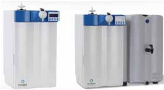
The LaboStar® 10 RO DI system has a small foot print and produces pure water with a quality of up to 10 MΩ-cm. The versatile system includes a 7 L storage tank with the option of adding a 30 l or 60 l tank. The pure water is collected in a tank and transferred by a built-in circulation pump. Typical applications are IC, Pathology, Buffer preparation, general chemistry, feed for laboratory ultra-pure water systems etc.
