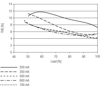
100 % load corresponds to the max. output power (full load) according to the table on page 2.
