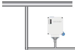
Installation under the pressure fitting
